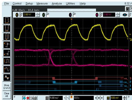
Figure 2: Six-channel measurement: Data line during a write trigger on RAS, CAS, WE, CS and CLK.
